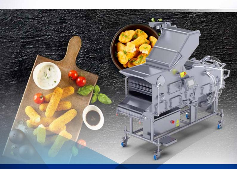
Application of all sorts of fine to coarse grains for high-quality product breading
